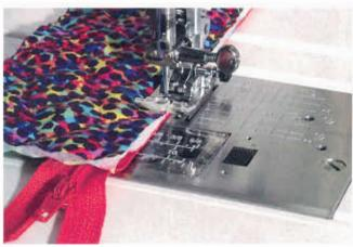
**2** Align the cut edge of the fabric with the edge of the zipper. Using the all-purpose foot riding against the zipper, and the needle to the far left position, stitch the length of the zipper.
