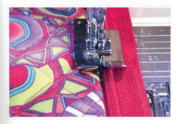
3 Fold the fabric over to expose the zipper coil. Position the edge-stitching foot with the bar between the zipper coil and the fold of the fabric. Move the needle position slightly left of the fold, and stitch across. Place the zipper pocket on another layer of center panel fabric, and trim to match.
